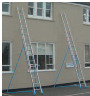
2. STABILISERS IN POSITION
